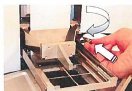
Figure 30 Fitting the transport lock of the tip comb holder
